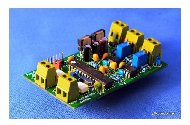
This board houses two low speed PWM to 0-10V analogue converters with optical input isolation and common output ground. It is suitable to interface devices with low frequency PWM (TTL level) outputs, such as flow meters, anemometers, etc, to standard variable frequency drives (VFD) or similar devices that require analogue input set-points to control an operational parameter (i.e. speed, torque, etc.).
